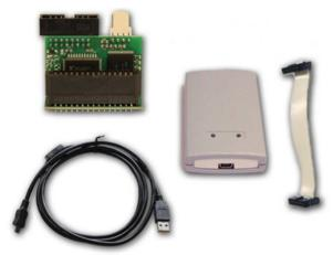
The J3 Chip is a module that plugs onto the J3 port of the Ford EEC. When plugged in to the J3 connector the Chip will disable the internal Ford tune and use the tune on the J3 Chip. The Chip is very simple to use and install. In order to program a Chip you will need to have a programmer, J3 Chip, Ribbon cable, and USB cable.
