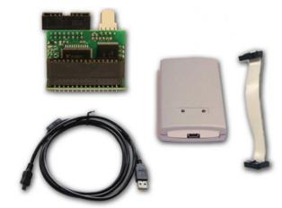
The J3 Chip is a module that plugs onto the J3 port of the Ford EEC. When plugged in to the J3 connector the Chip will disable the internal Ford tune and use the tune on the J3 Chip. The Chip is very simple to use and install. In order to program a Chip you will need to have a programmer, J3 Chip, Ribbon cable, and USB cable.
